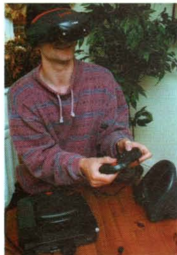
The first shot of the complete Virtuality HMD with infra-red tracking device
